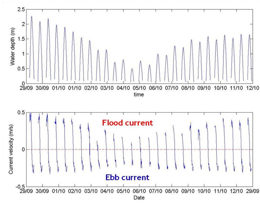
Figure 4.3: Water depth and current velocity measured over a spring-to-spring tidal cycle on Aunemouth Sands. The data were collected using a Valeport electromagnetic current meter and were collected at 4 Hz for 1 minute every 10 minutes. Positive current velocities denote flood currents and negative velocities represent ebb currents.
