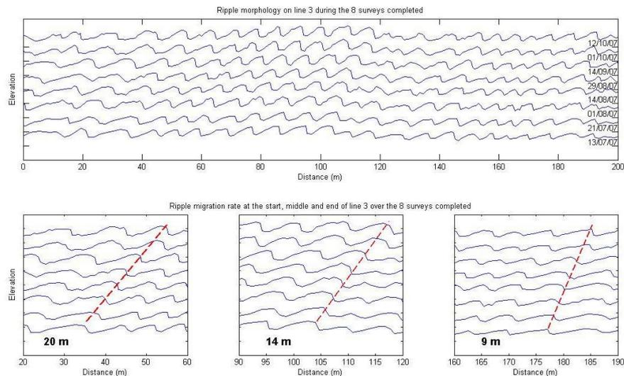
Figure 4.2: Results of sand wave monitoring on Aunemouth Sand from July to September 2007. The upper panel shows 8 consecutive surveys, vertically offset, taken at approximately fortnightly intervals. The lower three panels show zoomed-in versions of the data and clearly demonstrate that the sand waves migrate up-estuary. The bold numbers in the lower panels represents the estimated migration rate over the 3-month survey period.
